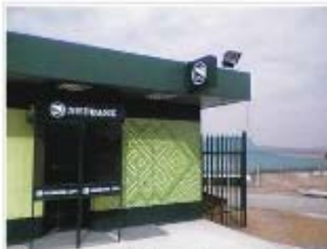
Flex face signs with powder coated aluminium frames
